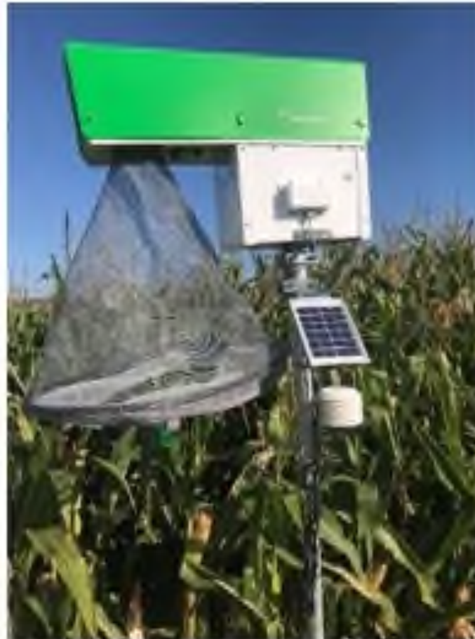
Figure 3: Trapview electronic trap for monitoring of corn borer
