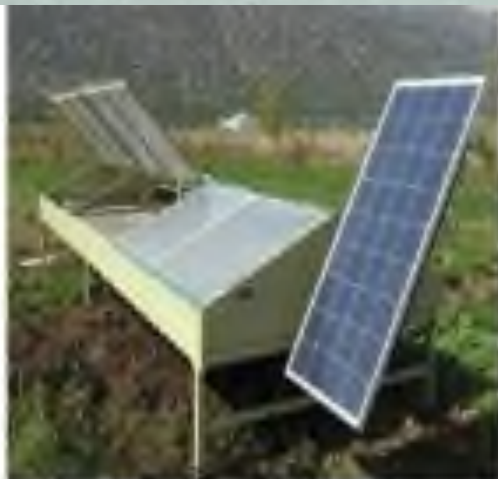
PV-powered solar dryer
