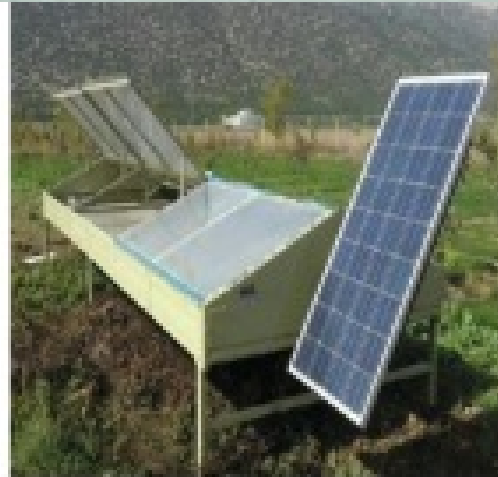
PV-powered solar dryer
