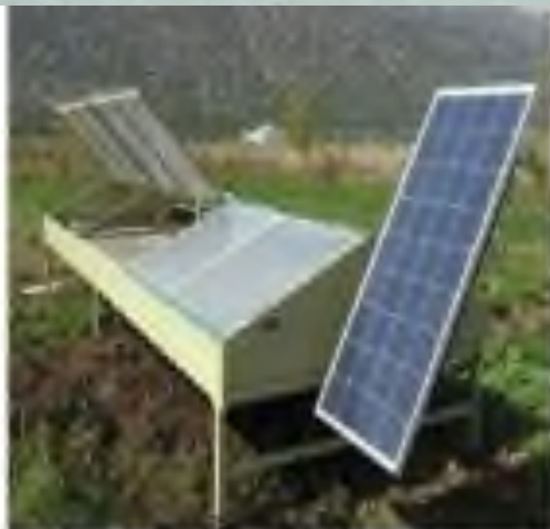
PV-powered solar dryer
